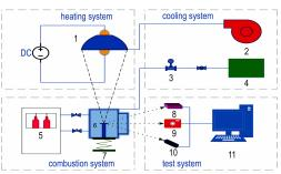
The ignition test of nano-aluminum/RDX mixture samples at different pressures was carried out using a medium-pressure condenser heating experimental bench. The high speed photographer, two-color infrared thermometer and fiber optic spectrometer were used to study the ignition characteristics and combustion process of the samples. The flame morphology, temperature and emission characteristics of the samples were analyzed in detail.
