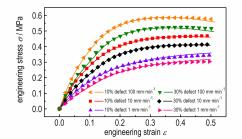
axial tensile and multi-step relaxation tests of HTPB propellants were conducted. Then, the parameter M was introduced as a function of strain and strain rate into the Ogden model and the visco-hyperelastic constitutive model of HTPB propellants without defects was established. At last, the damage factor f was implied to establish the visco-hyperelastic constitutive
