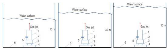
1—rocket engine, 2—thrust stand, 3—thrust sensor, 4—base, 5—pressure sensor, 6—lifting platform
