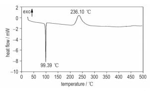
Fig.1 DSC curve of PrNQ at a heating rate of 10 ℃ • min<sup>-1</sup>
