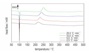
Fig.3 DSC curves of PrNQ at different heating rates
