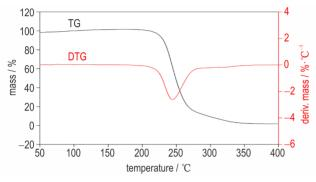
Fig.2 TG-DTG curve of PrNQ at a heating rate of 10 ℃•min<sup>-1</sup>
