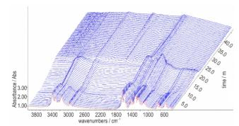
**Fig.4** *In-suit* FTIR spectroscopy of PrNQ at heating temperatures
