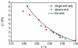
Non-local van der Walls correction was used to calculate the equation of state of TATB crystal. The result was found to be in good agreement with the experiment data. Based on the calculated results, the equation of state and vibration properties of TATB crystal at pressure of 0 GPa to 8.5 GPa were studied. The vibration modes were reassigned. Mode coupling and intermolecular interaction were analyzed.
