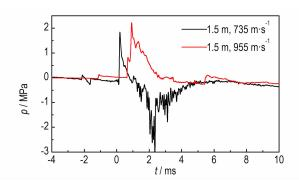
ZHOU Jie, HE Yong, HE Yuan, LING Qi Chinese Journal of Energetic Materials ,2016 ,24(11) : 1048-1056 Experimental study on shock initiation of simulative warhead was carried out. The blast air shock wave overpressure was measured, which act as a parameter to calculate the TNT equivalent.
