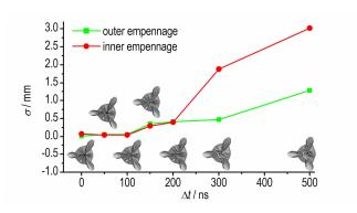
LI Rui, LI Wei-bing, WANG Xiao-ming, LI Wen-bin Chinese Journal of Energetic Materials ,2016 ,24(11): 1041-1047 The effects of three-point initiation synchronization error on formation and velocity of EFP with fins was studied by using LS-DYNA software in different condition. The asymmetric collision of detonation wave caused by the error and collapse of the liner were analyzed.
