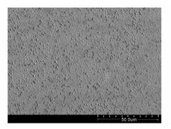
Ultrafine and spherical  $\varepsilon$ -CL-20 particles were prepared by the spray and ultrasound-assisted recrystallization device and characterized by SEM and XRD. Their thermal behaviors were studied by DSC.
