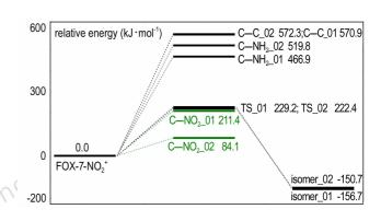
LI Xiao-dong, XU Zhe, WANG Jing-yu, WANG Xin-quan Chinese Journal of Energetic Materials, 2017, 25(1): 26-31 The complexes which were composed of charged particles and FOX-7 were optimized at the DFT-B3LYP/ 6-31++G (d, p) level and analyzed from the bonding styles and the electrostatic potential to study the effect of H<sub>3</sub>O<sup>+</sup> \OH<sup>-</sup> \NO<sub>2</sub> and NO<sup>+</sup> on the 1,1-diamino-2,2-dinitroethylene (FOX-7) dissociation channels.
