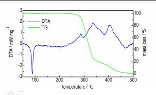
The structure of DNPwas characterized by optical microscope, FTIR spectrometer, UV VIS spectrophotometer, and TG/DTA thermal analysis instrument. The heat of detonation and detonation velocity of DNP were tested by an oxygen bomb calorimeter and the electrical measuring method. The detonation property parameters of DNP/CL-20 and TNT/ CL-20 composite explosives were calculated by the VLW program.
