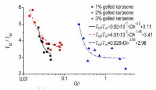
The temporal and spatial distribution characteristics of gelled kerosene were studied by using breakup experimental platform. The different breakup characteristics of kerosene and gelled kerosene were analysed. Relationship between  $T_{\rm tot}/T_{\rm ini}$  and Oh, and the variation tendency of streamwise and Cross-stream breakup region with the change of We number were investigated.
