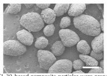
Four kinds of CL-20 based composite particles were prepared by slurry method using CL-20 as filler, wax and Estane5703 as desensitizers. Their crystal form, state of coating, thermal decomposition temperature and mechanical sensitivity were tested.
