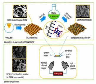
A new energetic composite was prepared compounding high-energy Hexanitro-2,4,6,8,10,12-hexaazaisowurtzitane (HNIW) into macroporous polyacrylonitrile (PAN) fibrosa by electrostatic spinning (ES) method and self-assembly method. The morphology, thermal property and combustion behavior of as-prepared composite were analyzed by SEM, FT-IR, thermal analysis and combustion residues analysis.
