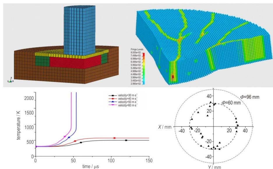
Taking Steven impact test as an example, a combined finite-discrete element method was established to simulate the crack growth and frictional heating in explosives. The history of load stress, crack distribution, temperature rise curve, ignition time and position, and velocity threshold of impact ignition were obtained.
