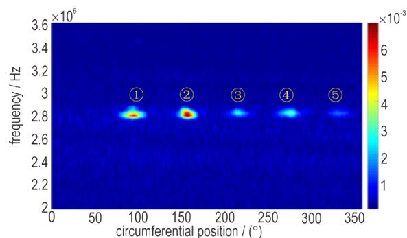
A new non-contact testing method based on electromagnetic acoustic resonance is proposed for the inspection of interface debonding defect in metal ring-energetic material bonding structure. Simulated of debonding defects specimen were scanned and imaged automatically with the developed automatic scanning system of electromagnetic acoustic testing.
