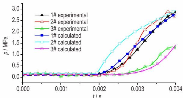
Ignition and transfer test of ignition charge in the propellant chamber was carried out in the structure of which the fire was ignited in the central tube and spread in the dense propellant charge bed. The propagation process of ignition flame was simulated. The experimental and simulation results were compared and verifying the correctness of the simulation model.
