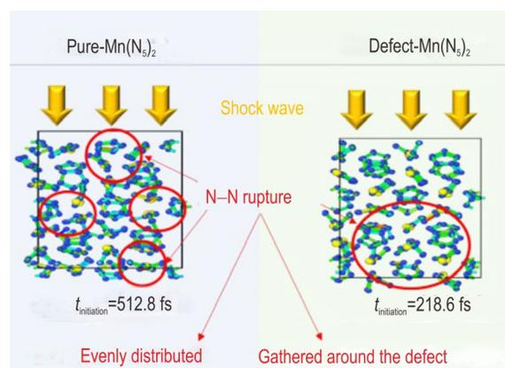
Chemical decomposition, and damage evolution of pentazolate salts, *ab initio* molecular dynamics method is employed to simulate the dynamics evolution and initial chemical reaction mechanisms for perfect  $\text{Mn}(\text{N}_5)_2$  crystal and the crystal with 3% vacancy defects under different shock velocities (8, 9, 10, 11, 12  $\text{km}\cdot\text{s}^{-1}$ ).
