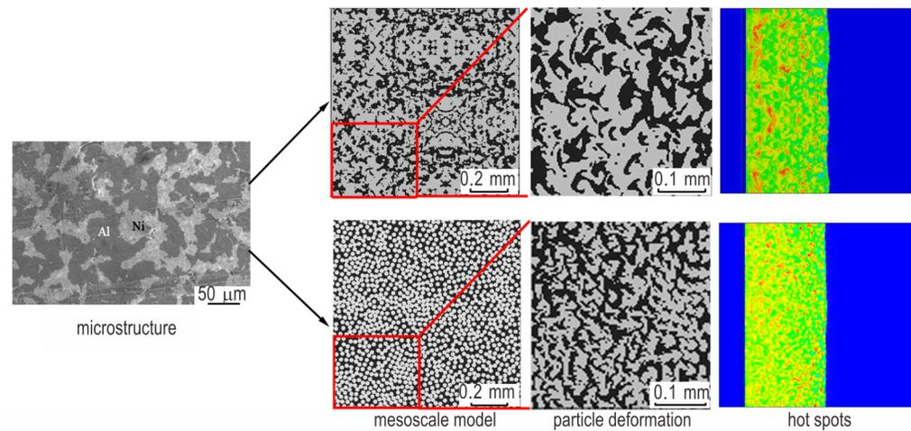
The dynamic behaviors of shocked Al/Ni energetic structural materials, including particle deformation, pressure, temperature, and propagation of shock waves, were investigated by two types of mesoscale modelling methods, which are established based on the SEM images and the uniform particle morphologies, respectively.
