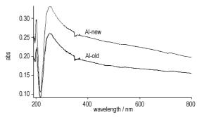
CHU Guang, TANG Yong-jian, CHU Shi-jin, WEI Jian-jun, LI Chao-yang, LIU Wei Chinese Journal of Energetic Materials, 2006, 14(3): 227 - 230 Al nanoparticles were prepared by flow-levitation method. The morphologies, granularities, structure and properties of particles were investigated by EDAX, XRD, UV-visible absorption spectroscopy and thermal analysis (DSC-TG) techniques.
