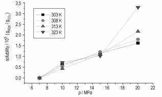
The solubility of RDX in supercritical carbon dioxide (SC-CO $_2$ ) at 303, 308,313,323 K and a pressure range of 7 – 20 MPa were measured.
