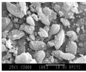
ε-HNIW was prepared by nitrolysis of two chemicals tetraacetyldiformylhexazaisowurzetane (TADFIW) and tetraacetyldibenzylhexazaisowurzetane (TADBIW) respectively. Thermal decomposition parameters and impact sensitivity ( $H_{50}$ ) of the two kinds of HNIW samples were determined and SEM pictures were given.
