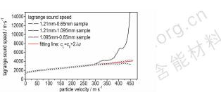
The dynamic response of hydroxyl-terminated polybutadiene (HTPB) samples solidified by toluene diisocynate (TDI) were investigated under ramp loading up to 1.2 GPa. The velocity response curves of three HTPB samples with different thickness were obtained by Photonic Doppler Velocimeter(PDV). The sound velocity vs. particle velocity curves and stress vs. specific volume curves were obtained by Lagrange analysis method.
